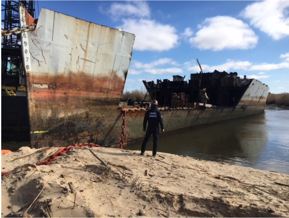
13 January 2018 - LCDR Brege observes the forward sections of the ship cut down to just above the waterline as the ship is being prepped for pulling onto the beach with the 300T chain puller.
