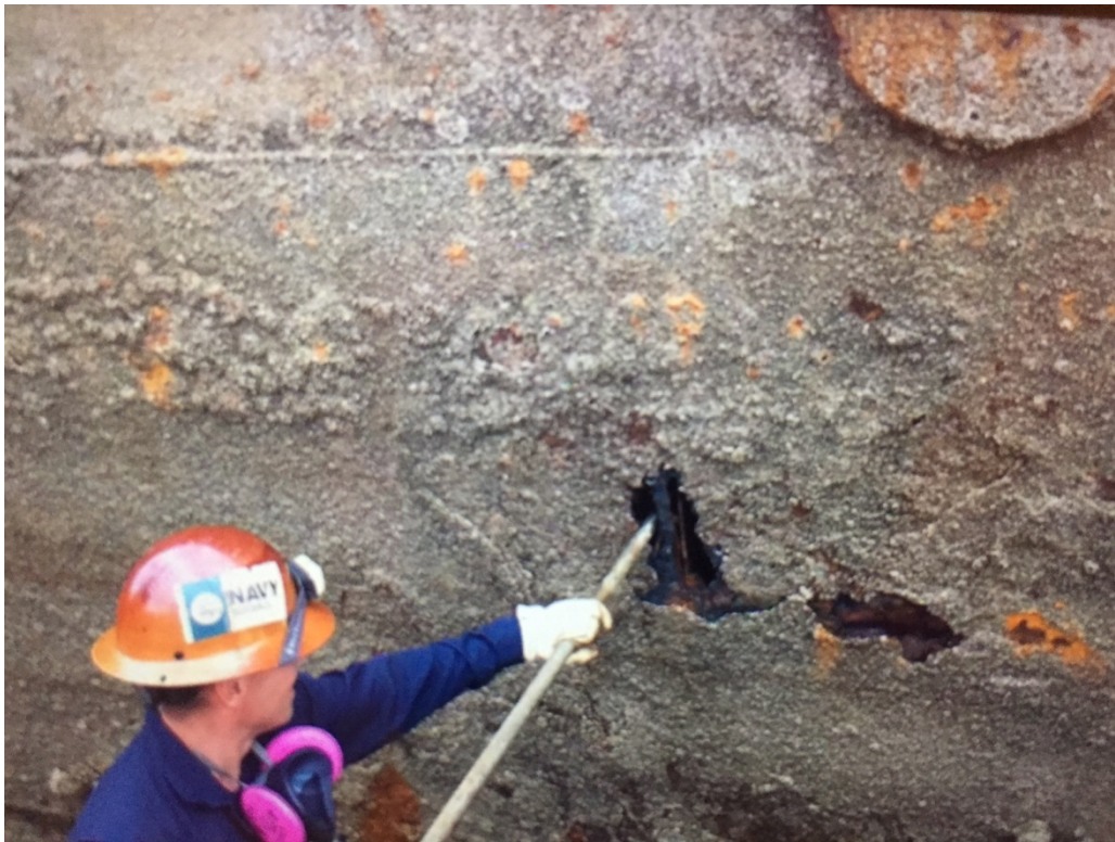
EX-SHADWELL's hull is easily pierced with just a metal rod, showing the severity of hull degradation
