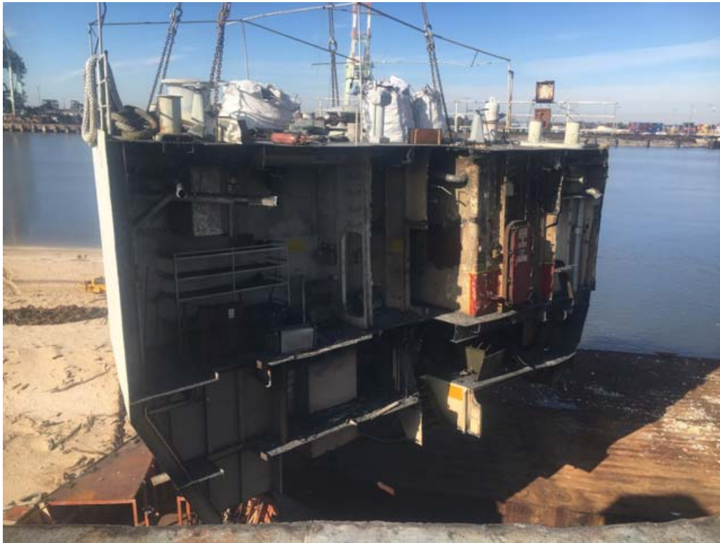
Bow section being lifted from SHADWELL's hull on 7 January. Note mooring line on left and anchor capstan center.
